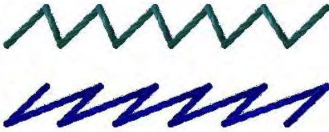
Two Steil segments, each having the identical stitch length and Steil angle. The short connection method has been applied in the top segment, and long connection method to the bottom one.
