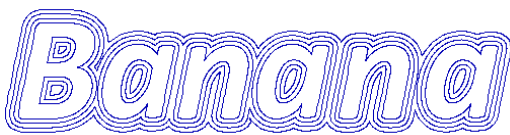
Above, offset with three repeats created with the "Merge offset shapes" set to on; below, same segment with this setting off.
