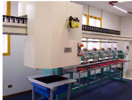
A Bridge Laser (SEIT Laser 4) machine connected with a Tajima multi head embroidery machine
