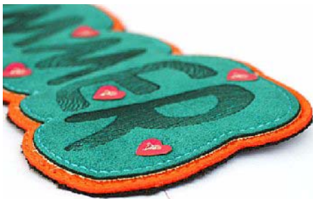
A design with laser fills. The text in the design are engraved using laser rays.
