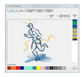
The dialog shows a preview of your design, the sequence of colors currently assigned to it along the right (the Needle Bar) and the color palette available on your machine along the bottom.
