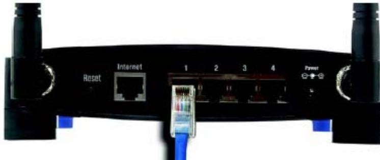
Tajima machines can coexist on your business network. If you wish to connect your business network to the Internet, connect an Ethernet cable to the port labeled Internet on the Wireless Router. Connect the other end of the Ethernet cable to your Cable or DSL Broadband Modem.
