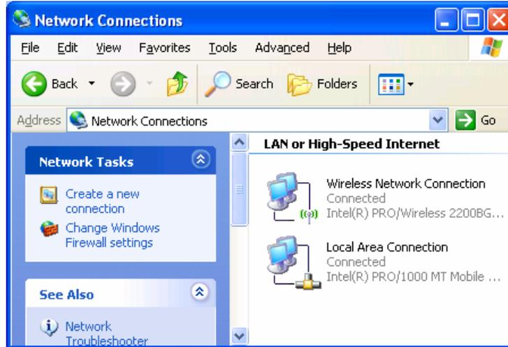
Check to make sure that the network adaptor that is used to connect to the router network where the embroidery machine is located is the only network adaptor connected. In the image above, two network adaptors are connected. To disable one of the network adaptors, right click on the network adaptors and select Disable. Make sure you are not disabling the adaptor that is used to connect to your embroidery machines. If only one network adaptor is connected, then no changes need to be made.
