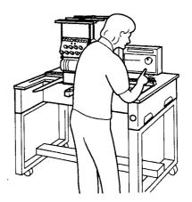
• Be sure to turn off the power switch before manually turning the main shaft.
